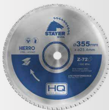
Disco Widia TGC, diente sandwich Ø 355x2.4x25.4 mm Z72
